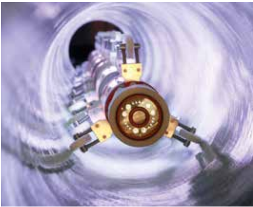
UV lamp trolley from Berolina for sewer pipe refurbishment
