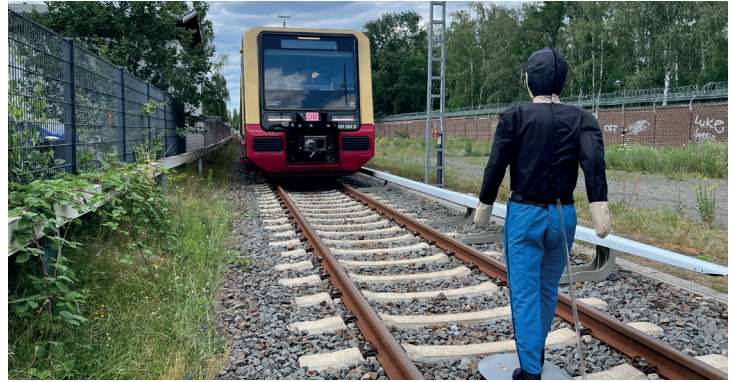
BerDiBa project – test of automatic obstacle detection
